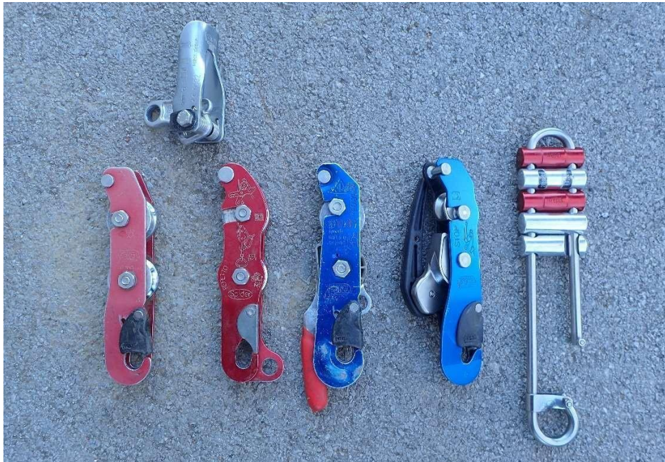
Figure 1: Different versions of descent devices
