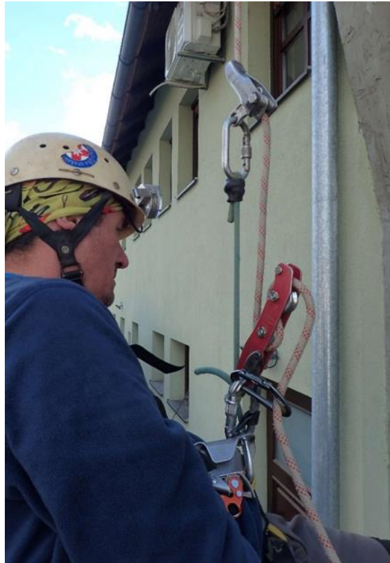
Figure 3: Injured Caver Hanging in a Shunt and Simple Descender
