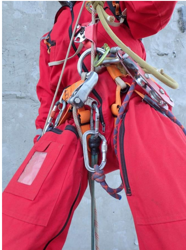
Figure 11: Crossing the Shunt Using the Knot Passing Method
