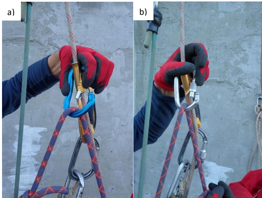
Figure 8: Working space of the carabiner at the upper opening of the blocker (Figure 8a: HMS carabiner; Figure 8b: oval carabiner)
