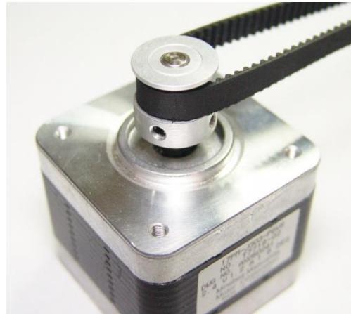
Slika 6.6. Motor NEMA 17 s remenicom i remenom
